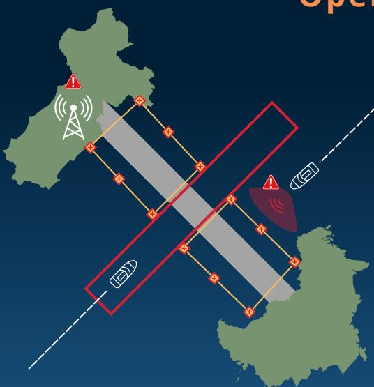
VA Protect employs an automated AIS messaging system to establish rules governing boundaries for specific areas. This system alerts marine traffic to hazardous zones at sea, safeguarding your assets from collisions, protecting people, and preventing damage to both surface and underwater assets.
